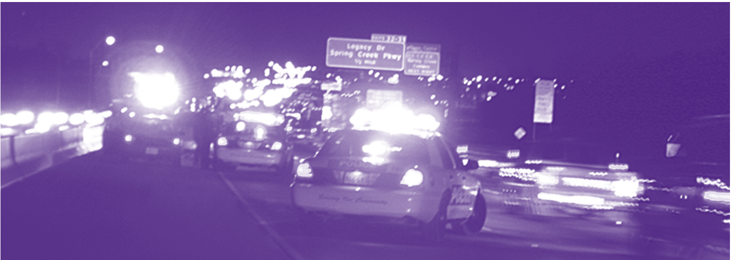
Emergency warning lights should be minimized as conditions warrant. More is not always better.
