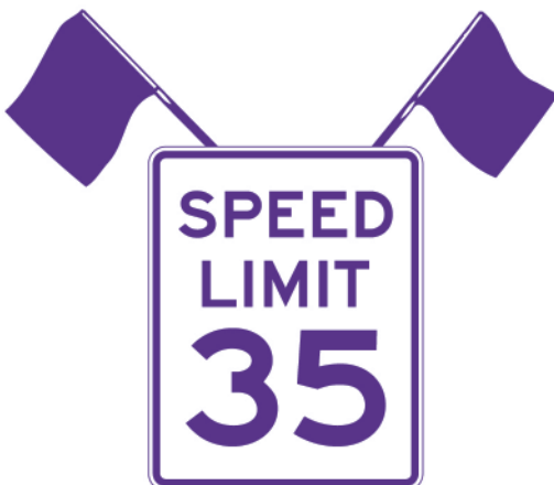
Red / orange flags call attention to a change in the posted speed limit.
