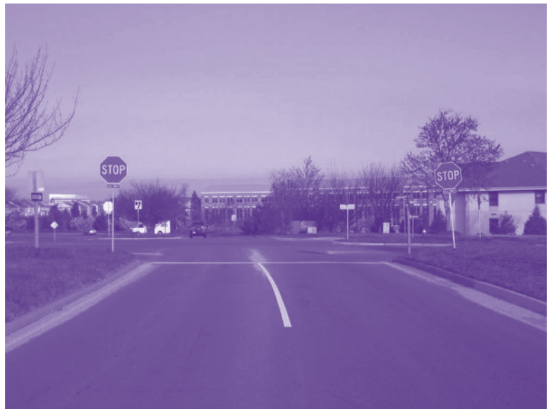
Figure 3: Additional, larger (30-inch) stop signs with stop bars
