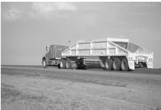
When reshape is finished, good quality surface gravel should be placed quickly before rain causes subgrade to lose its shape.
