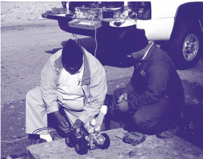
Ronald Bettis is setting up the Rover ® by hooking up the power and video controls
