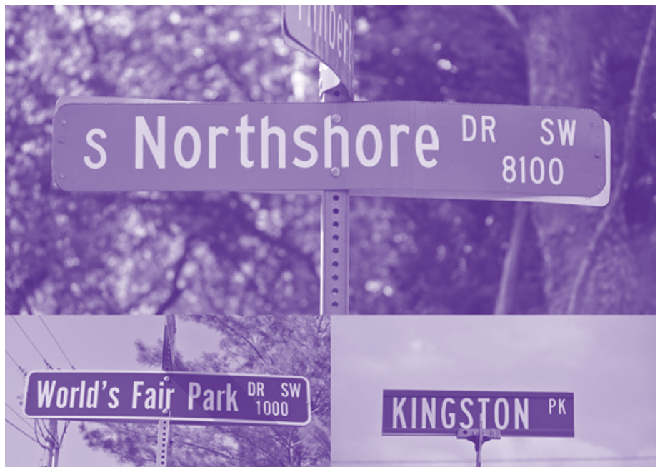
These signs show three of the four available color options for street name signs, including the standard white on green (top), white on brown (lower left), and white on blue (lower right).
