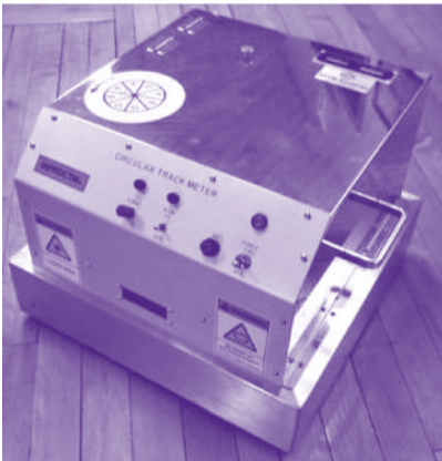
© APTech – The Circular Texture Meter uses a laser-displacement sensor to measure the vertical profile of a pavement surface.
